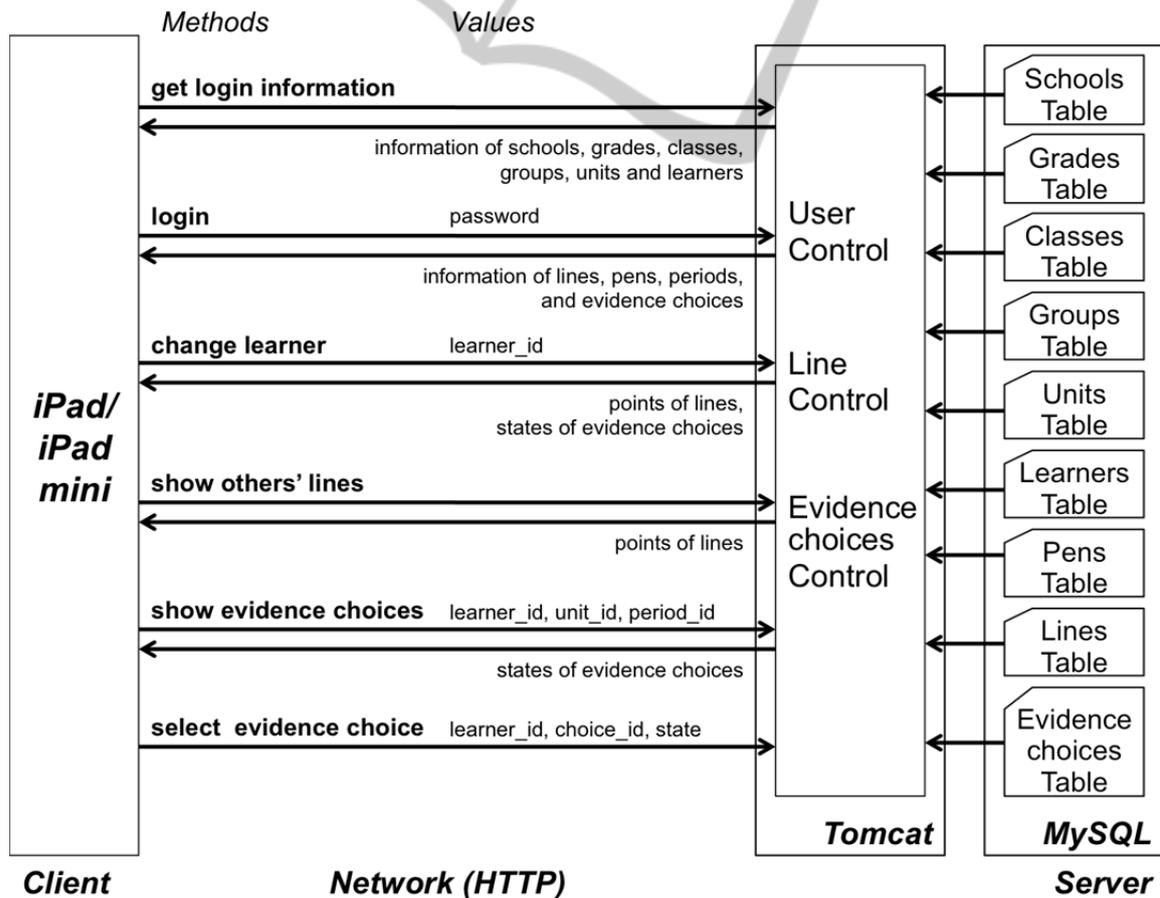
Figure 1: The system configuration.
