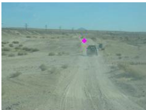
Figure 1: Vanishing point detection in all type of environment, although without any lane marking.
