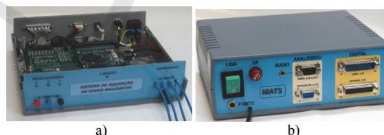
Figure 1: The designed box to accommodate the acquisition system board. a) Front view with cover open; b) Back view.
