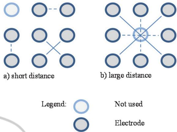
Figure 4: Scheme of distributing the pair of electrodes (bipolar) oriented every 45° with different distances between electrodes. a) Short distance b) Large distance.
