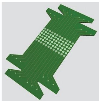
Figure 11: Prototype of flexible sensor array for detection of motor unit activity.
