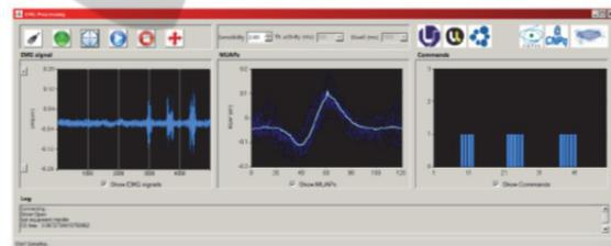
Figure 9: Graphical interface illustrating sequences of action potentials extracted in real time and translation of them into commands (Júnior, 2013).
