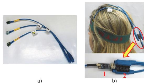
Figure 5: a) Set of sensor arrays used to capture EMG signals from facial muscles. b) Set of sensor arrays in use by an individual. The signal conditioner and digital converter circuit (1) and the connector (2) are highlighted.
