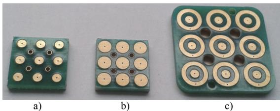
Figure 3: The three sensors array designed. a) Circular sensor array (diameter of 2mm and distance between electrodes (DE) of 4mm); b) Circular sensor array (diameter of 3mm and DE of 4mm); c) Concentric sensor array (internal diameter of 2mm, external diameter of 6mm and DE of 7mm).
