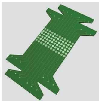
Figure 11: Prototype of flexible sensor array for detection of motor unit activity.
