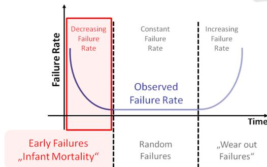
Figure 1: The bathtub curve describes the life stages of semiconductor devices.
