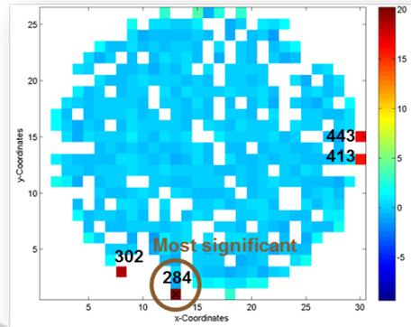
Figure 10: The wafer map represents the resulting NNR calculation on source 3 (see Figure 9) with 8 neighbors (NNR8). Device 284 is the most significant one.
