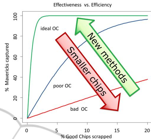
Figure 5: With ever smaller devices, a distinction between good devices and Mavericks becomes challenging. Therewith, the efficiency of currently applied screening methods decreases. New methods are expected to counteract. Consequently, the steeper the operating curve, the higher the classification power of the method.
