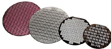
Figure 2: Wafers can be distinguished e.g. regarding the size and number of devices, which is considered with NNR.
