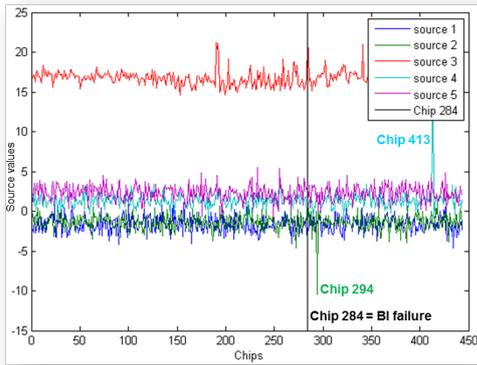
Figure 9: With a quadratic de-mixing matrix  $W$  the dimension of the resulting sources remains the same. Source 3 (red) is conspicuous compared to the remaining sources and is therefore assumed to contain the most information. Source 2 and 4 show one peak each and thus will be investigated in more detail.
