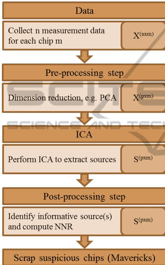
Figure 7: The flowchart provides an overview of the proposed way of proceeding.
