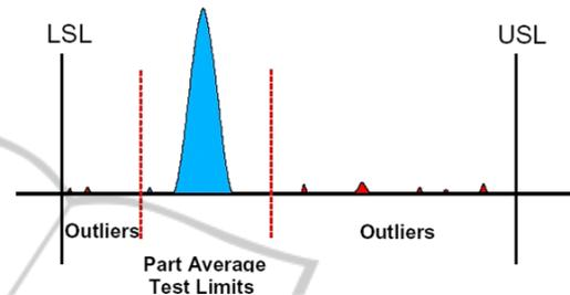
Figure 3: PAT limits, marked in red, are more severe than the lower (LSL) and upper (USL) specification limits.
