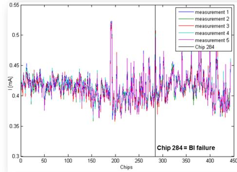
Figure 8: Each IDDQ measurement can be visualized as a signal over all devices. This figure shows the first 5 (superimposed) IDDQ measurements taken from overall 577 available, used as a dimension-reduced basis for the following ICA.
