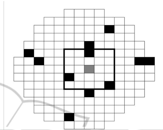
Figure 6: To calculate the NNR value for each device (here marked in gray), just the pass devices are taken into account because for the electrical fail devices (marked in black) no value is available. The black square shows the involved devices for a 24-based neighborhood.
