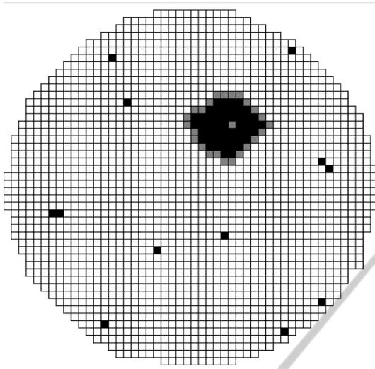
Figure 4: Good devices surrounded by bad devices (marked in black), are inked out (marked as gray devices).
