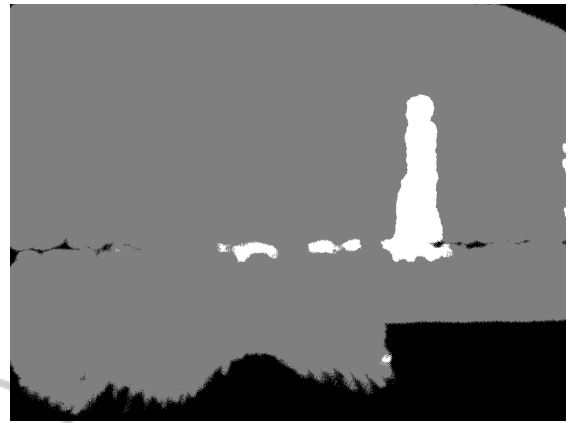
Figure 10: An image corresponding to the thresholded probability field B_k . Gray is static, White zone need to be inpainted and Black is unknown because there is not enough neighbors.
