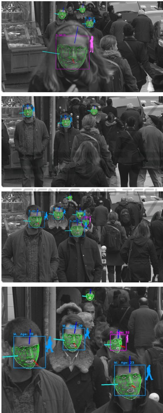
Figure 6: Results in outdoor conditions: face tracking, pose estimation, age and gender estimation (test video n°1).
