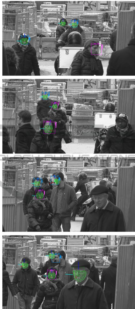
Figure 7: Results in outdoor conditions: face tracking, pose estimation, age and gender estimation (test video n°2).
