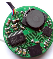
Figure 1: Electronic unit used for on-board processing of the sensor signal with wireless interface for data transfer via radio frequency identification (RFID).
