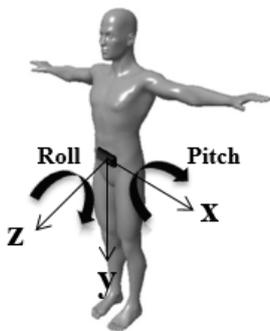
Figure 1: Definition of the sensor axis.
