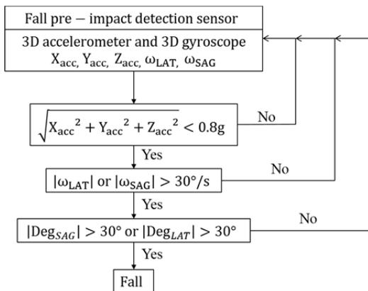
Figure 4: Pre-impact fall detection algorithm.
