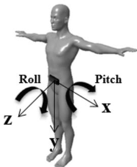
Figure 1: Definition of the sensor axis.
