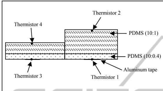
Figure 1: Device Structure.
