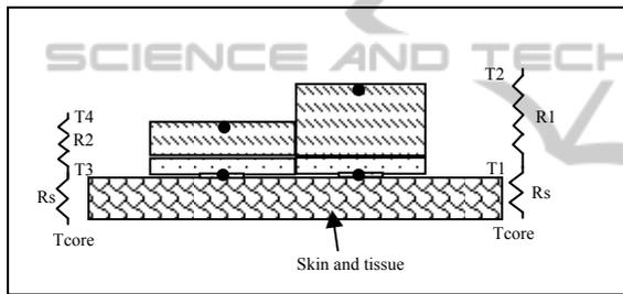
Figure 2: Schematic of device placed on skin and analogous equivalent circuit with two parallel heat flow channels and thermal resistances network.
