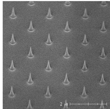
Figure 3: SEM image of the plasma etched nanoelectrode array.
