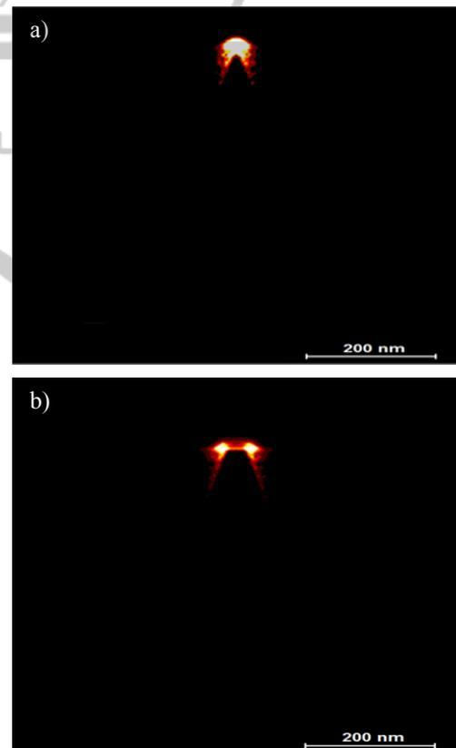
Figure 4: Simulation of the electric field gradient  $\text{grad } |E|^2$  above the nanoelectrodes with a) 10 nm and b) 50 nm tip diameter. Maximum field gradient (white) is close to the tip.
