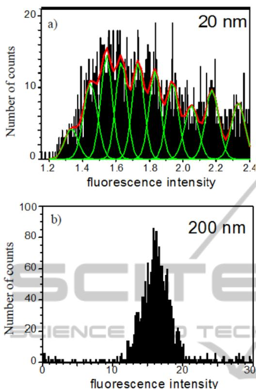
Figure 7: Fluorescence intensity distribution of dielectrophoretically immobilized polystyrene nanospheres. Bead diameters are a) 20 nm and b) 200 nm. Electrode diameter is 50 nm. a) For particles smaller than the electrodes, accumulation of approx. 1 to 15 particles per electrode tip occurs. b) 200 nm spheres are immobilized as singles.
