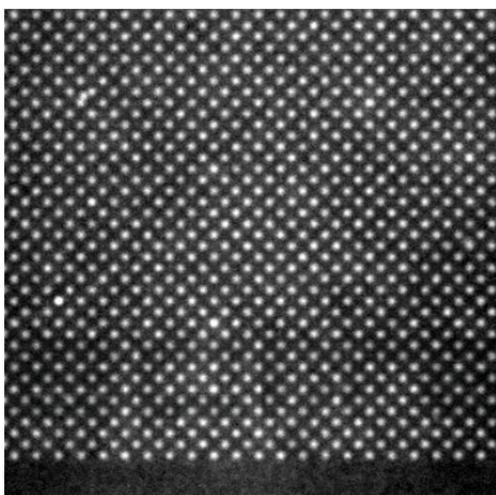
Figure 5: DEP field induced immobilization of the fluorescently labeled protein BSA on nanoelectrodes after field application of 10 kHz and 7  $V_{RMS}$  for 10 min.
