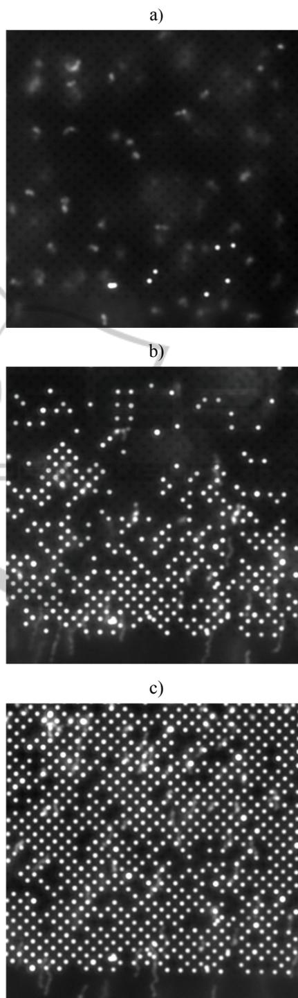
Figure 6: Top view microscopic images through the transparent top electrode of 200 nm fluorescent polystyrene nanospheres in water on the nanoelectrode array. a) Before field application, b) after field application at 17 kHz and 8  $V_{RMS}$  for 12 s and c) after 60 s field application.
