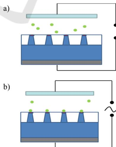
Figure 1: Dielectrophoresis: Schematic illustration of the experimental setup. a) Nanoobjects are suspended in water b) By applying inhomogeneous AC electric fields, electrical forces act on polarizable particles. These forces lead to a local particle accumulation. Distance between top electrode and electrode surface is about 100  $\mu\text{m}$ .
