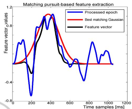
Figure 3: The figure depicts how each single feature vector is extracted from the preprocessed epoch (blue). Matching pursuit selects the best matching Gaussian atom. The atom that was selected in the first iteration is depicted in red. To get the feature vector (plotted in black), element-by-element multiplication of the epoch with the selected Gaussian atom was calculated.
