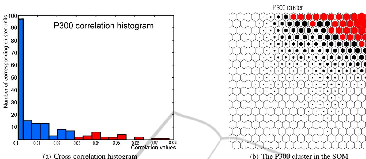
Figure 6: The histogram illustrates how the normalized Gaussian function scaled to resemble the P300 component correlates with the SOM codebook vectors. The threshold was set to 0.03 and any cluster units that were associated with higher correlations were tagged as the P300 component candidates (in red). Fig. 6(b) shows the distribution of the P300 candidates on the map. The cluster units in red belong to the P300 component cluster.
