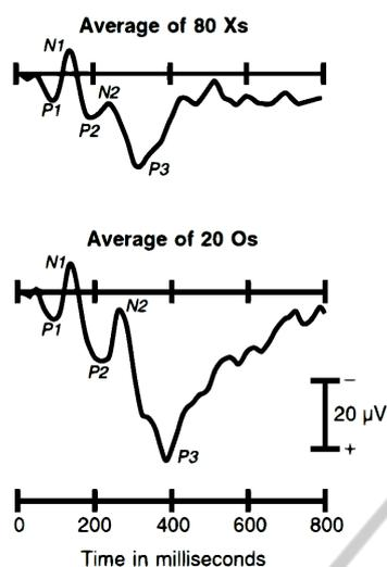
Figure 1: Comparison of averaged EEG responses to nontarget stimuli (Xs) and target stimuli (Os). The ensemble averaging is necessary, otherwise the event-related potentials could hardly be distinguished from noisy EEG signal. There is a clear P3b component following the Os stimuli. Negative is plotted upward (Luck, 2005).
