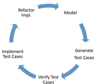
Figure 3: The formal test-driven development cycle.
