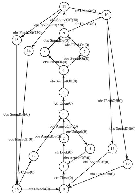
Figure 6: The second partial model of the CAS capturing only one trace to the armed state and all the traces afterwards.
