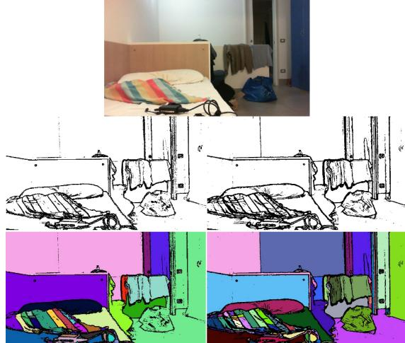
Figure 2: Image segmentation and component labelling. The right pair of images shows our approach (using a 11x11 median filter and threshold value of 21), while the left one shows the result using Sobel operator. Our implementation manages to separate more regions.
