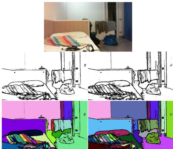
Figure 2: Image segmentation and component labelling. The right pair of images shows our approach (using a  $11 \times 11$  median filter and threshold value of 21), while the left one shows the result using Sobel operator. Our implementation manages to separate more regions.
