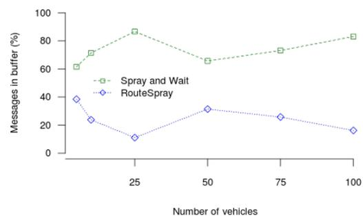
Figure 4: Improvement in the buffer occupancy by spray technique.
