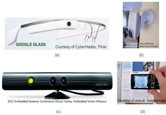
Figure 2: Examples of vision embedded systems (a) Google Glass (b) Security Camera (c) Kinect. Xbox Game Console (d) Text Reader on a mobile phone.
