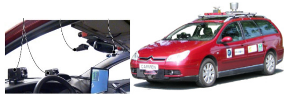
Figure 1: MINARDA system and CARMEN car- Ready for simulation driving as well as naturalistic driving data collection.
