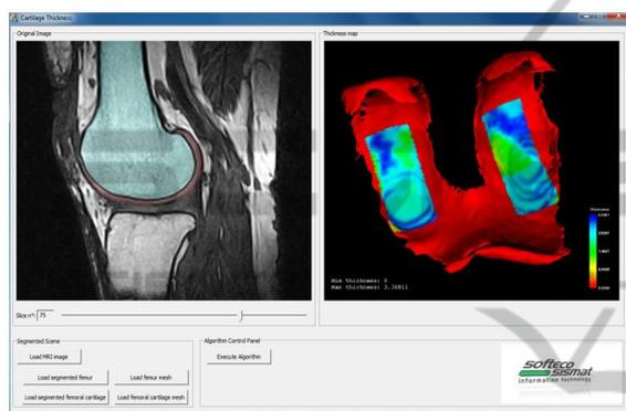
Figure 3: Tool for measuring the femoral cartilage thickness near the weight bearing regions.
