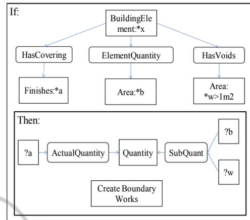
Figure 2: A Conceptual Graph of Quantity surveying rule.
