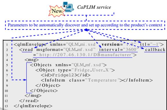
Figure 3: Automatic self-setting of the QLM parameters.
