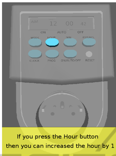
Figure 4: Picture of a plug-in timer in the virtual environment with the “present” operation
