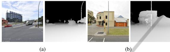
Figure 4: Example pairs of co-registered intensity and depth images (a) Image and depth map of an intersection. (b) Image and depth map of building.
