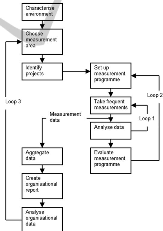
Figure 2: the new three-loop QTM process.
