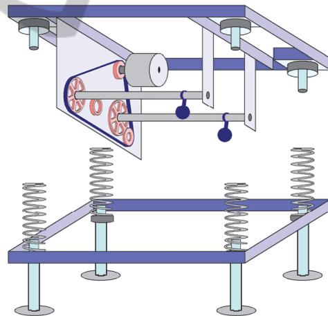
Figure 2: Schematic of the vibrating table.
