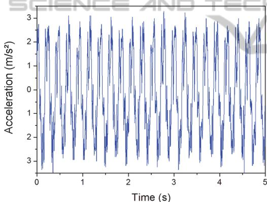
Figure 5: Example of z-axis signal issued from accelerometer (Acc-W) located on wheelchair frame.
