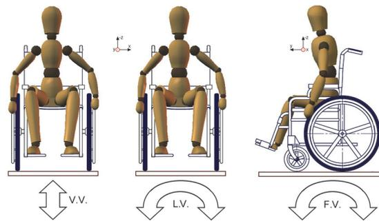
Figure 1: Basic vibrations that can be induced on a manual wheelchair: vertical vibration V.V, lateral vibration L.V and fore-and-aft vibration F.V.
