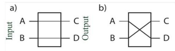
Figure 1: Cross-bar switch: a) Bar configuration, b) cross configuration.
