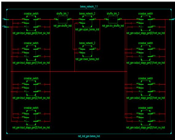
Figure 6: Schematic of Beneš network with  $N = 8$ .
