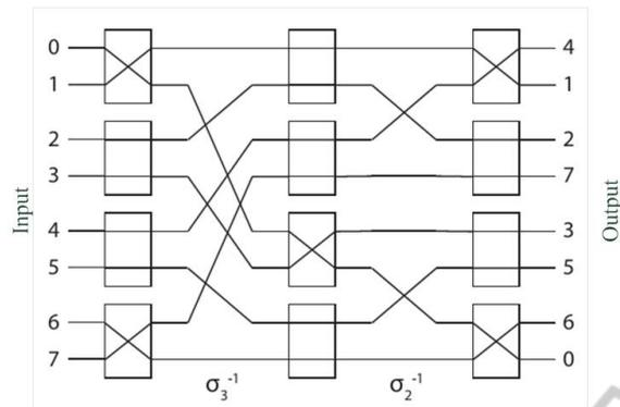
Figure 2: Baseline network for N=8, [Aust13] [AR10a] [AR10a].
