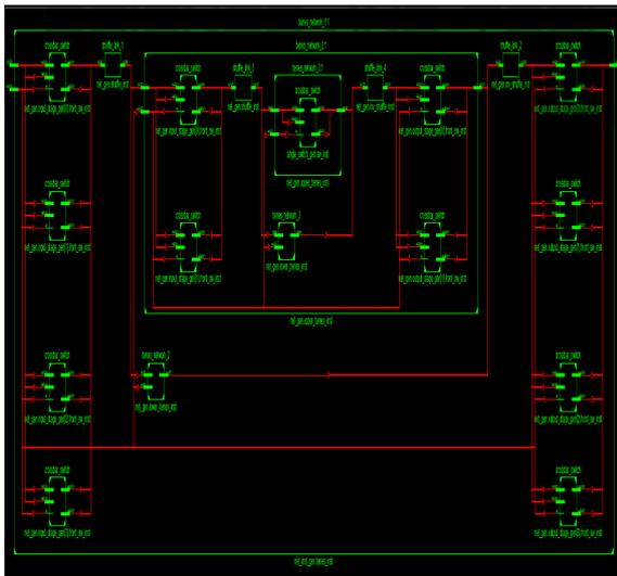
Figure 7: Partly expanded schematic for Beneš network with  $N = 8$ .
