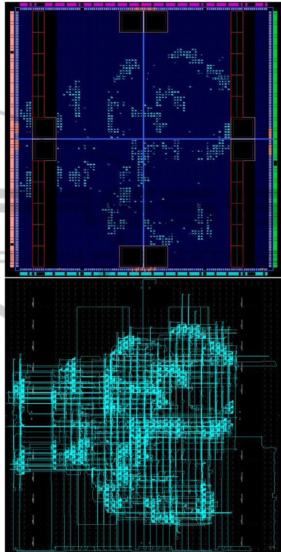
Figure 8: Place (top) and route (bottom) results for Beneš network with  $N = 8$ . Device: Xilinx xc3s700an.
