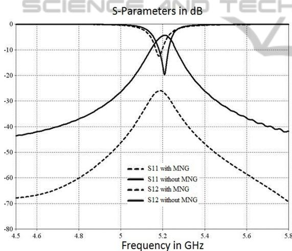
Figure 2: Simulated S-Parameter for both cases (with and without MNG).
