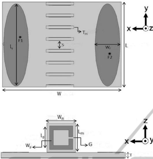
Figure 1: Two-element antenna array based on elliptical patch radiating elements with MNG. Top view (top) and side view (bottom).
