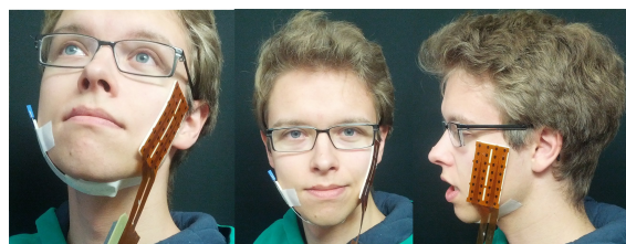
Figure 1: Positioning of the EMG array during recording. One 4 \times 8 array is affixed to the speaker's cheek and one 1 \times 8 array is affixed underneath the chin. Image taken from (Wand et al., 2013b) with permission.
