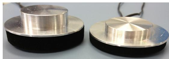
Figure 2: Front view of the two prototypes. Radii of the two prototypes are 22.0 mm, while heights are {15.0, 9.0} and {8.0, 5.0} mm, respectively.
