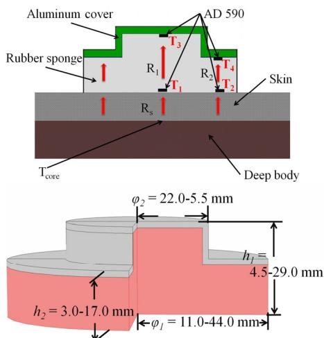
Figure 1: Upper: The illustration of the two-layer structure and the arrangement of the four temperature sensors (AD 590, Analog, 2-pin style). It is supposed that the heat from deep body part flows as the arrow's indicating and no transverse heat flow arises in the skin and the thermometer. Lower: The cross-section view of the thermometer. The thickness of the top aluminum cover is 1 mm.
