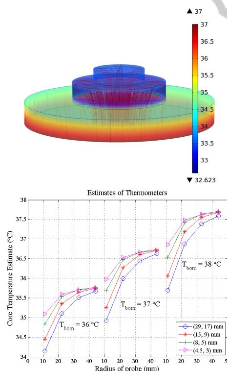
Figure 4: Upper: An image of temperature distribution and heat flow inside the prototype. Lower: Results of the simulations. X-axis is the radius of the thermometer; Y-axis is the estimates of thermometers.
