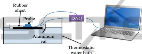
Figure 3: The schema of the experimental system.
