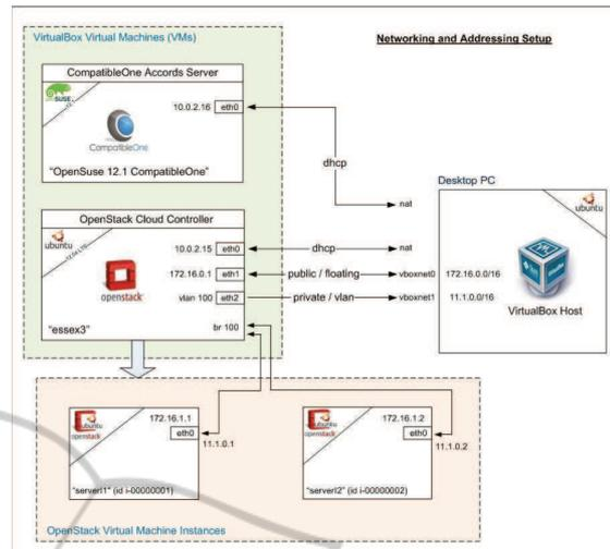
Figure 6: OpenStack and CompatibleOne Architecture
