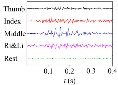
Figure 6: Example of different patterns of finger flexion motions' sEMG signals. Ri&Li represents the ring & little flexion motion.
