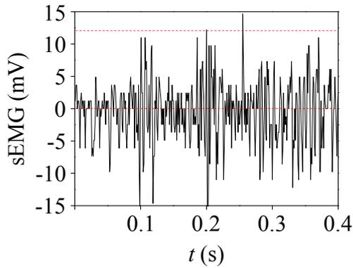
Figure 8: Example of the rest position's signal, which indicates the amplitude of noise. The red and dashed lines show the *MINPEAKHEIGHT* of 12 mV.
