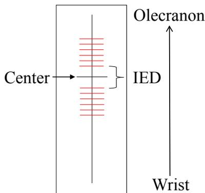
Figure 3: Placement of pair of electrodes on forearm for IED experiment. The center of the two electrodes is on the midline of the forearm's palmer surface, and at 0.75 of the distance from the wrist to the olecranon. The IED increases from 30 to 80 mm at an interval of 10 mm.
