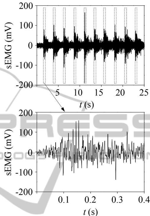
Figure 2: Example of sEMG signals' segmentation process. Each window size in the figure at the top is 400 ms. The signal segmented in the bottom figure shows that it also contains the muscles' contraction signal.
