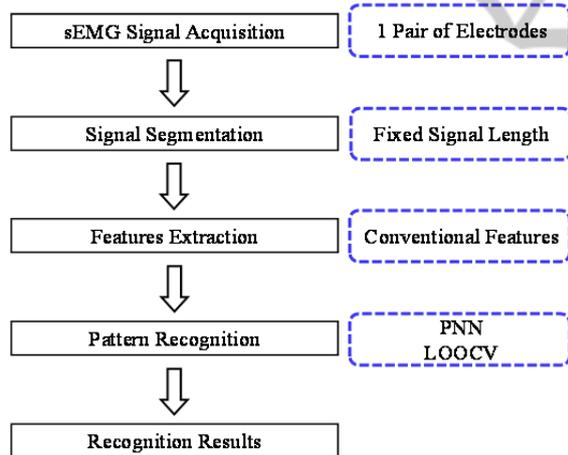
Figure 1: Conventional recognition methodology of IED experiment.
