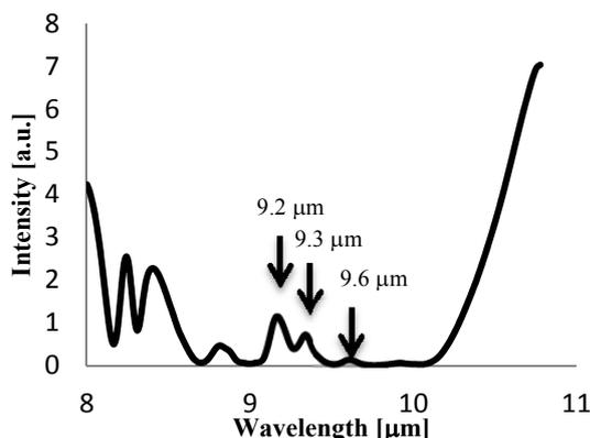
Figure 1: D-glucose spectrum that were measured by FTIR spectroscopy in a KBr sample. The spectra show the characteristic peaks between 8  $\mu\text{m}$  to 10.5  $\mu\text{m}$ .
