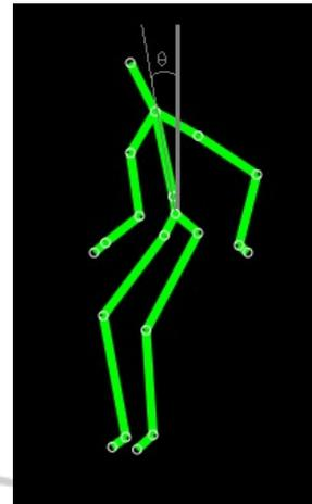
Figure 3: Trunk angle calculation.
