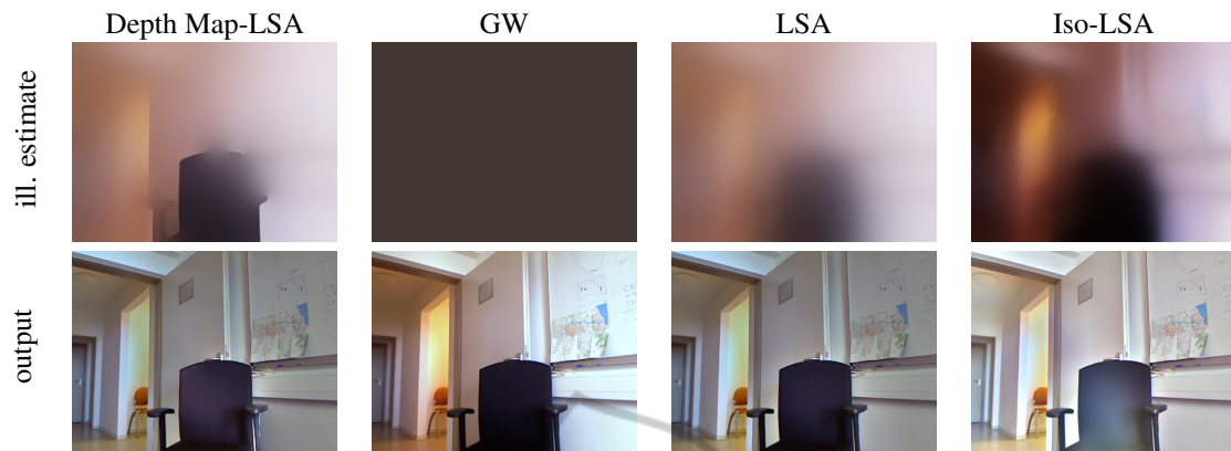
Figure 6: Comparison with three other color constancy algorithms for image 2: gray world assumption (GW), local space average color (LSA), computation of anisotropic local space average color along iso-illumination lines (Iso-LSA).
