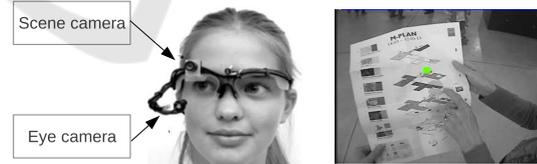
Figure 1: Left: illustration of a mobile eye-tracker consisting of a scene camera and an eye camera. Right: output of a mobile eye-tracker in which the data of the scene camera and the captured gaze point (green dot) are combined.
