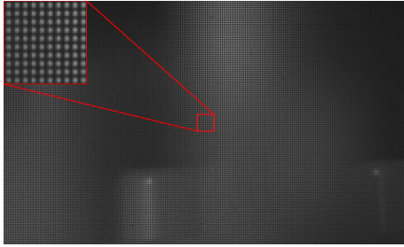
Figure 8: Image taken by opening all the pixels in controllable aperture.
