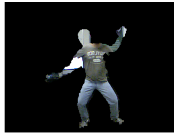
Figure 6: Kinect performs asynchronous acquisition of RGB and depth images. As a result, the quality of the RGB-D alignment procedure performed by Kinect’s API can be affected by rapid movements of the user, which leads to inconsistent RGB-D image formation.
