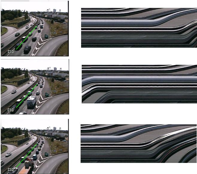
Figure 5: Examples in which traffic congestion has been automatically detected.
