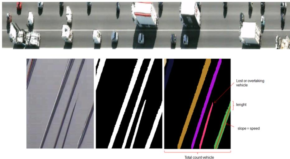
Figure 1: Top: 1-D segment perpendicular to the circulation lanes. Bottom: 1-D segment parallel to the circulation lane. Horizontal axis: temporal axis. Vertical axis: Segment axis.
