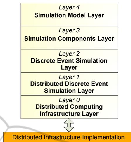
Figure 1: SimArch layered architecture.
