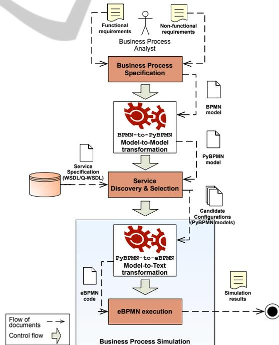
Figure 3: Model-driven BP simulation method.
