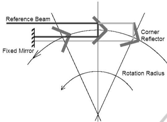
Figure 1: Long path scanning algorithm.
