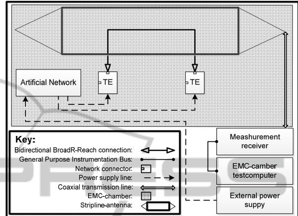
Figure 2: Blockdiagram of the test environment. Two Technica/tinytron media converter are connectet with each other to interchange Idle-Codes.
