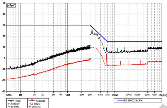
Figure 4: Result of the emission measurement. Blue: Limit line from GS 95002; Black: Peak detector result; Red: Average detector result.
