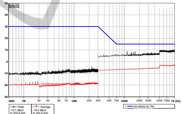
Figure 3: Baseline noise floor meashurement. Blue: Limit line from GS 95002; Black: Peak detector result; Red: Average detector result.
