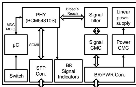
Figure 1: Block diagram of a Technica/tinytron optical Ethernet-to-BroadR-Reach media converter.
