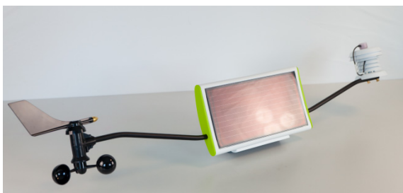
Figure 1: A GreenBee with weather sensors. Ozone, particulates and noise sensors are behind the solar panel.
