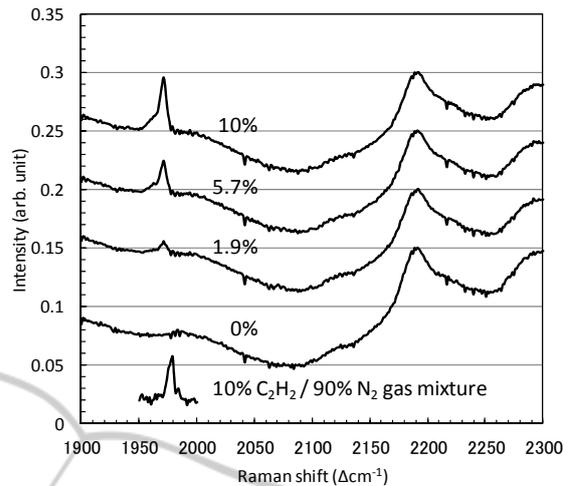
Figure 3: Raman spectra of  $\text{C}_2\text{H}_2$  gas at different concentrations dissolved in the insulation oil.
