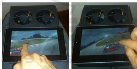
Figure 1: Drag interface being used while viewing a 360° video. Wind accessory coupled with the tablet.
