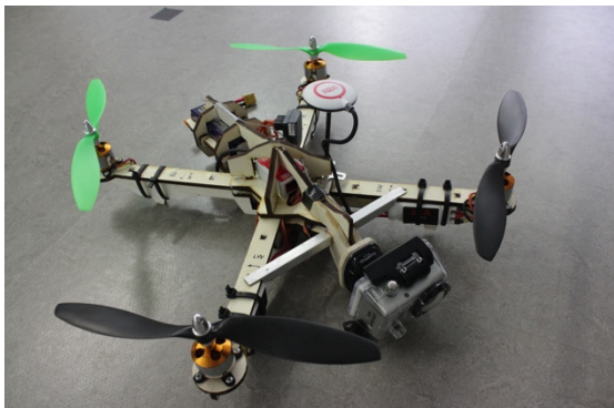
Figure 5: The whole copter made by beech plywood.
