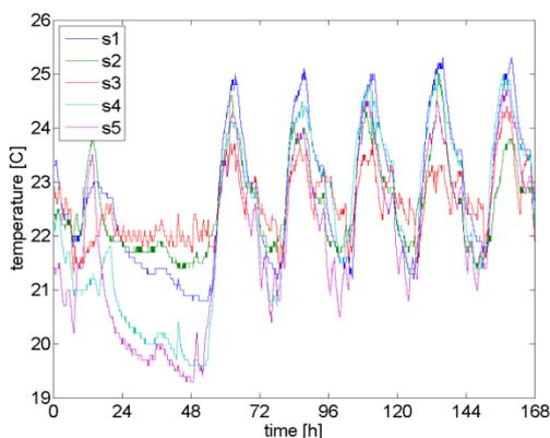
Figure 1: Temperature record at five candidate locations of the sensor net nodes. The screening data was recorded in course of one week, starting from Sunday.
