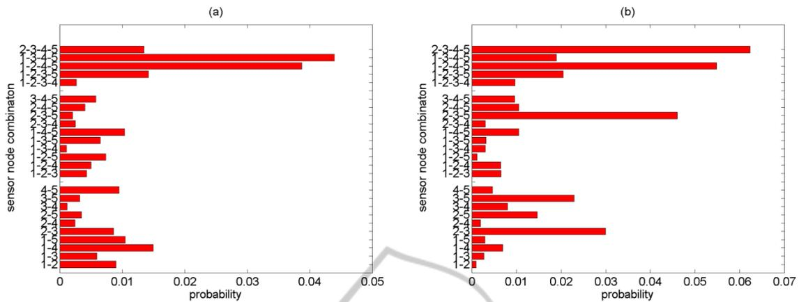
Figure 5: Probability of providing the messages loaded with maximum uncertainty and minimum mutual information on: (a) temperature, (b) relative humidity, using different combinations of sensor net nodes.
