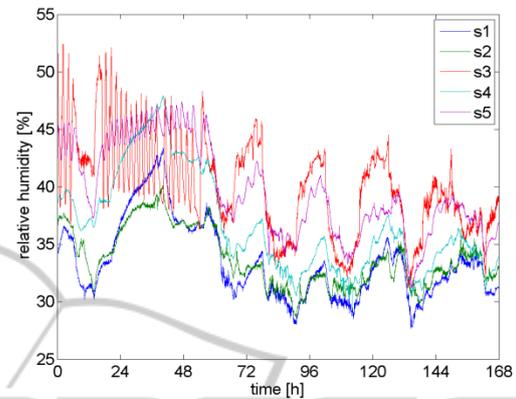
Figure 2: Relative humidity record at five candidate locations of the sensor net nodes. The screening data was recorded in course of one week, starting from Sunday.
