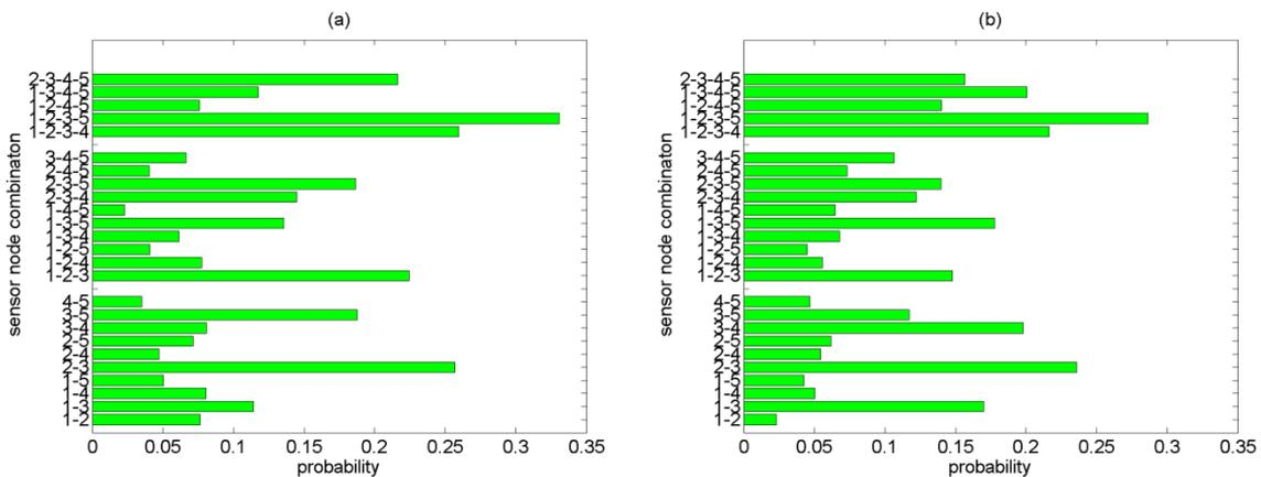
Figure 4: Probability of providing the messages on indoor air humidity loaded with: (a) maximum uncertainty, (b) minimum mutual information, using different combinations of sensor net nodes.
