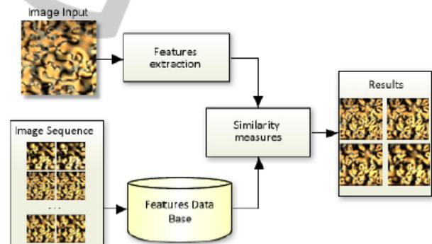
Figure 7: The proposed method to identify the phases of liquid crystal.
