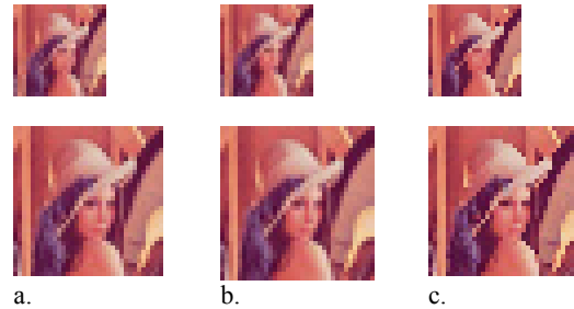
Figure 6: 1/25 and 1/15 block decimation for Lena (2x scale): a) block mean, b) bicubic interpolation and c) block median.
