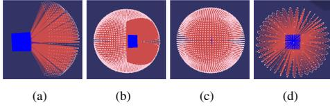
Figure 1: One camera location with 6 frustums:  $\psi = 0^\circ, \theta = 0^\circ, 90^\circ, 180^\circ, 270^\circ$  respectively;  $\theta = 0^\circ, \psi = 90^\circ$  and  $270^\circ$  respectively.  $\phi = 0^\circ$  for all. (a): 1 frustum; (b): the other 5 frustums; (c): 6 frustums with high resolution images; (d): 6 frustums with low resolution images.
