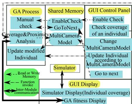
Figure 5: GUI Tool functionalities and framework.
