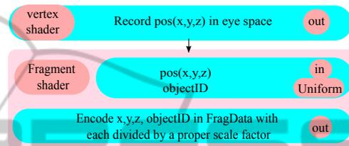
Figure 2: Vertex and fragment shader programming.
