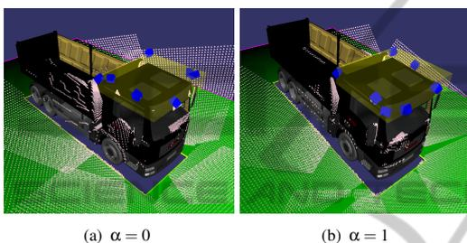
Figure 8: Camera locations of the optimal layouts: (a) Proximity = 0.39(m), (b) Proximity = 0.21(m).
