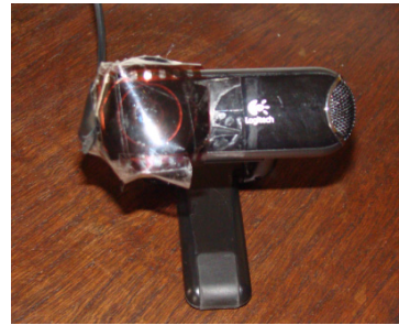
Figure 6: Modified web camera used to do hand veins acquisition.
