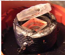
Figure 4: Square Infrared filter that needs to be removed in order for the webcam to capture infrared images.
