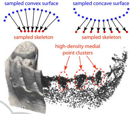
Figure 3: Relationship between local surface curvature and medial cloud density. **Top:** Concept sketched in 2D. **Bottom:** High-density point clusters are formed inside positive-curvature 3D surface areas (front teeth).
