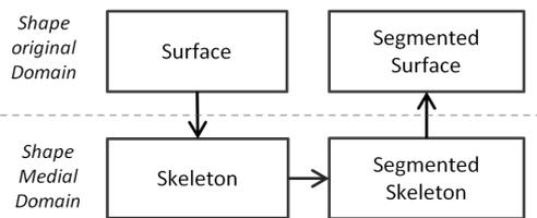
Figure 1: Algorithm workflow: A shape is transformed into the medial domain. Its skeleton is next segmented by a mean-shift approach. The segmentation is transferred back to the original shape.
