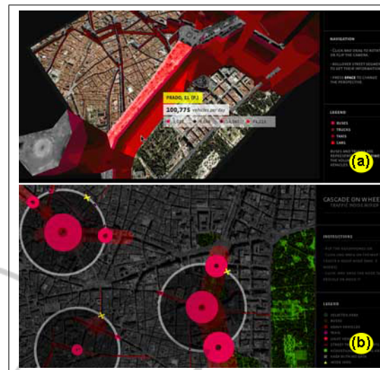
Figure 1: (a) Walls Map Piece - a 2D/3D map with walls representing streets with dense traffic. The greater the flow of vehicles in a street segment, the higher the corresponding part of the wall. (b) Traffic Noise Mixer. Audible noise is produced in order to indicate the amount and types of vehicle in selected regions. Courtesy of (Thirion et al., 2008).
